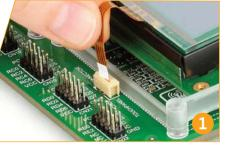
Figure 13-1: Put Touch Panel flat cable in the connector
