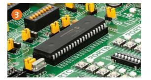
Figure 4-5: Properly placed microcontroller will have equally leveled pins.
