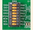
**IMPORTANT:** In order to use PWM backlight both **SW4.5** and **SW4.6** switches must be enabled at the same time.
