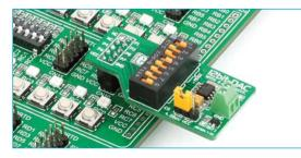
Figure 10-5: IDC10 male headers enable easy connection with mikroElektronika accessory boards
