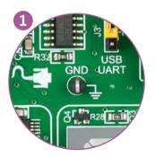
Figure 20-1: 3 oscilloscope GND pins are conveniently positioned so each part of the board can be reached with an oscilloscope probe
