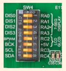
NT: In order to use PWM backlight both SW4.5 and SW4.6 switches must be enabled at the same time.
