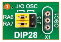
Figure 4-6: RA6 and RA7 as I/O pins (when using internal oscillator)
